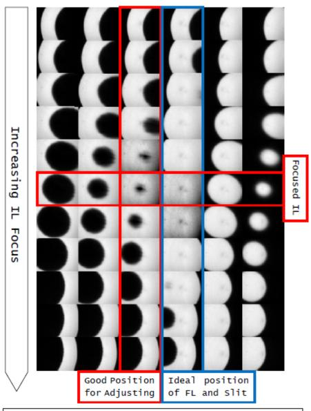
Condition: TEM Spot 1/Alpha 3, Magnification x10k, Slit width 20eV
